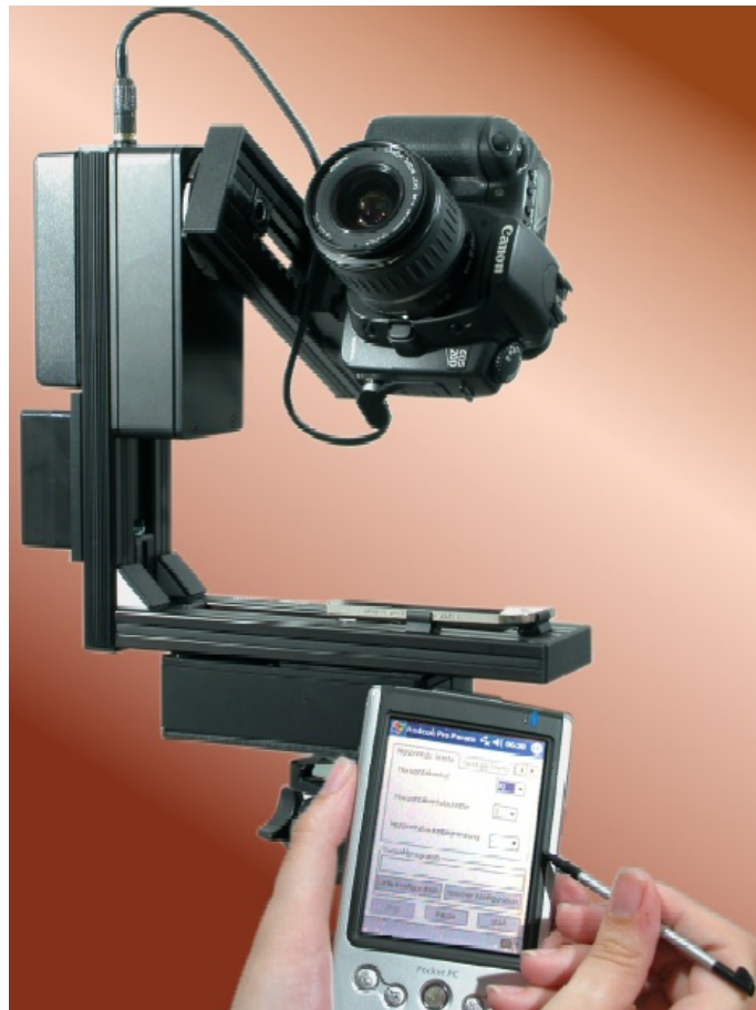
Figure 7.4: Automated panorama head. (Source: Wikipedia https://commons.wikimedia.org/wiki/File:Rodeon_vr_head_01.jpg )
